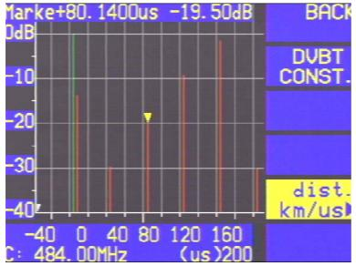
By means of the impulse response representation, it is possible to measure echoes in the transmission path or multiple path reception. The green line (on the left in the screen to dB) represents the received used carrier. The other (red) lines are echoes. For multiple path reception, pre-echoes can also occur, if an unwanted transmitter has a shorter distance to the receiver as desired.
